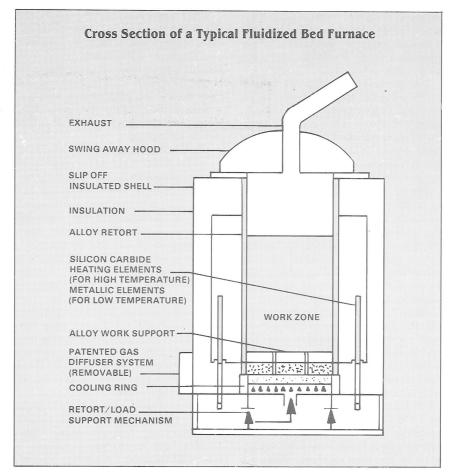
simple in design and operation, the fluidized bed furnaces house a bed (a container, or retort) containing very dry, uniformly sized particles of inert aluminum oxide. Air or blends of gases for specific treatment processes are introduced through a diffusion plate beneath the retort, separating and mobilizing the minute particles to give them fluid-like characteristics. Silicon carbide elements, between the retort wall and the furnaces's outer insulated wall, heat the flowing particles.
